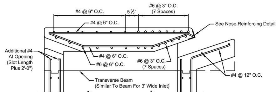
PARTIAL SECTION - 4'-0" THROUGH 6'-0" INLET WIDTH
