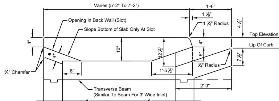
PARTIAL SECTION - 4'-0" THROUGH 6'-0" INLET WIDTH
