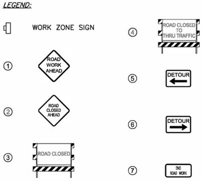
TEMPORARY ROAD CLOSURE - CHESTWOOD AVE. FROM TAMARACK AVE. TO SPOONWOOD DR. DURING TIMES OF CONSTRUCTION, PROVIDE TRAFFIC CONTROL AND SIGNAGE IN ACCORDANCE WITH FDOT INDEXES TO ADEQUATELY PROHIBIT TRAFFIC FROM ENTERING THE DESIGNATED WORK AREA (SMALL SECTION OF BOTH LANES OF CHESTWOOD AVENUE TO REMAIN CLOSED). AT ALL OTHER TIMES, TWO LANES TO REMAIN OPEN. CONSTRUCT TEMPORARY DRIVING SURFACES AS NECESSARY. MAINTAIN SEPARATION OF PEDESTRIAN TRAFFIC AT ALL TIMES.
