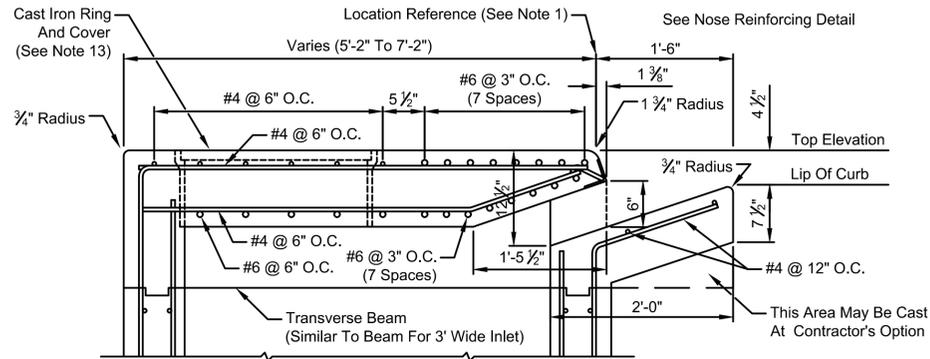
PARTIAL SECTION - 4'-0" THROUGH 6'-0" INLET WIDTH
